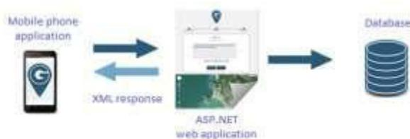
Figure 2: Geostep architecture
