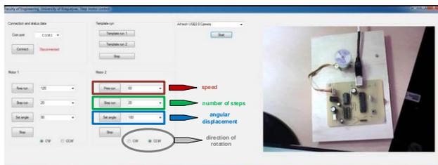
**Image 5:** The user interface for remote experiment with stepper motor [7]
