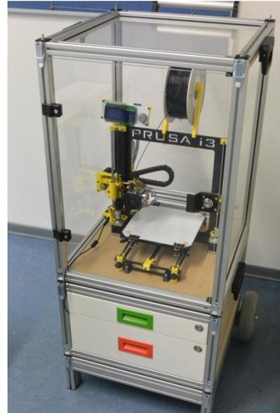
**Image 5:** Modular trolley with 3D printer
