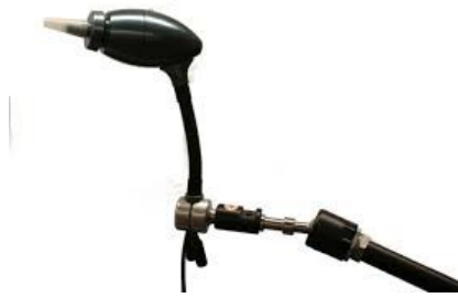
Image 5: Mouth-controlled mouse emulator. [17]
